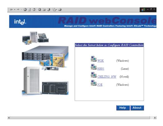
A RAID server or a client system that does not have a RAID controller installed can be used to remotely manage a RAID server through a standard Web browser interface. To do this, point the browser at the registration server using either the host name or the IP address of the registration server, such as <a href="http://w2k:3570">http://w2k:3570</a> or <a href="http://w2k:3570">http://w2k:3570</a>.
